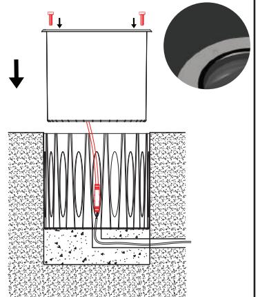
Connect the main power cable to the cable of the luminaire with the use of an IP68 connector or special insulation material. Install the lamp body of LED inground light and fix the recessing box and lamp body by screws.
