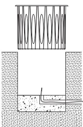
Open the hole for the fixture to be mounted. After preparing the drainage, fill the hole with gravel up to 20-30 cm considering a provision for power cable. To check the drainage, pour a bucket of water into the open pit and make sure that the water is drained within 15-20 minutes. Take attention with the position level being careful to place a suitable drainage bed.
